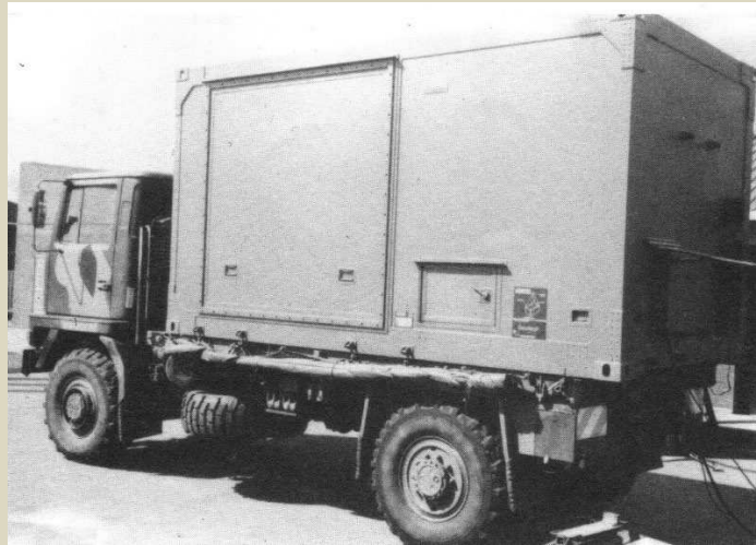
Figure 106. TACIPRINT based upon a container carried on a 8-tonne flatbed truck
