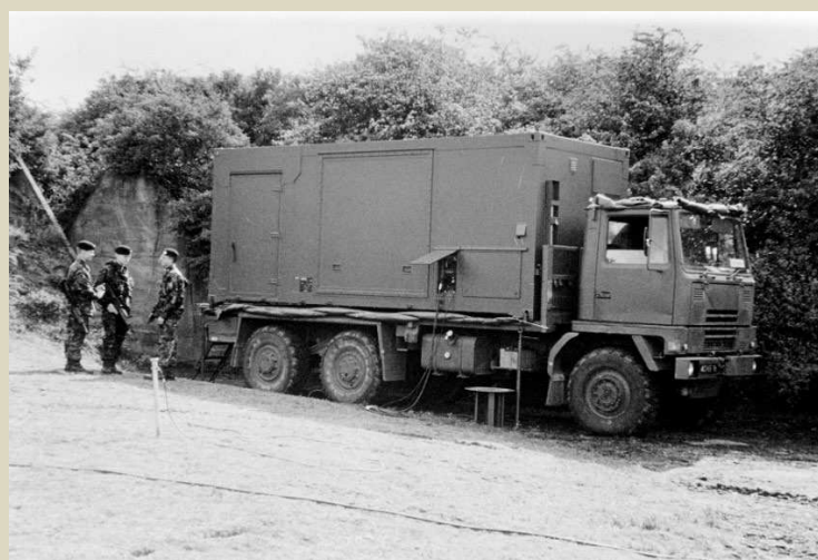
Figure 105. Geographic Support System based upon a container carried on a 10-tonne flatbed truck
