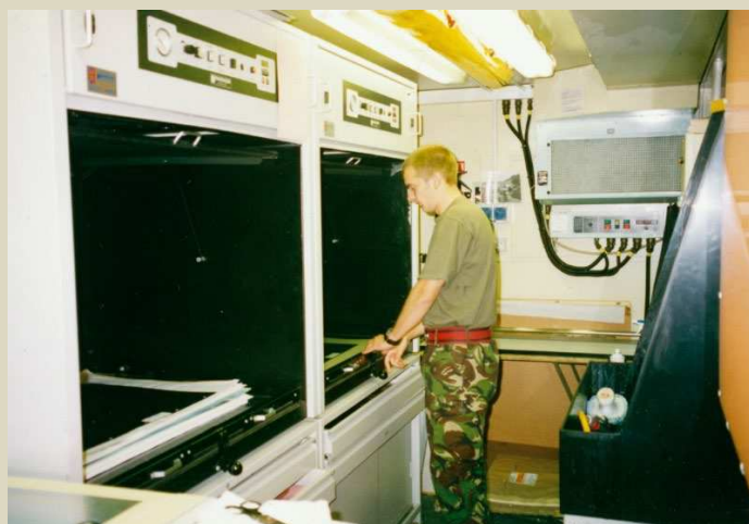
Figure 111. Helio container with printing plate exposure frames and printing plate developing sink
